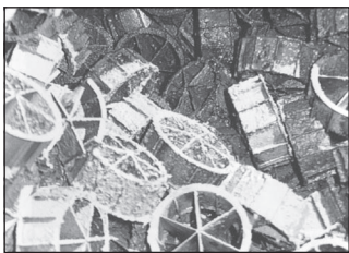
Figure 1.21 Plastic Media. The secondary sedimentation tanks are filled with these little objects. They provide a very large surface area on which bacteria can grow
